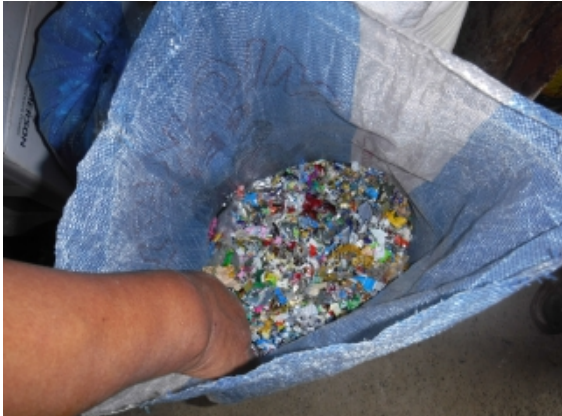
Illustration 20: Shredded plastic can then be easily ecobricked.
